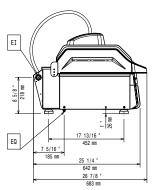
Electrical inlet (power) Electrical Outlet
